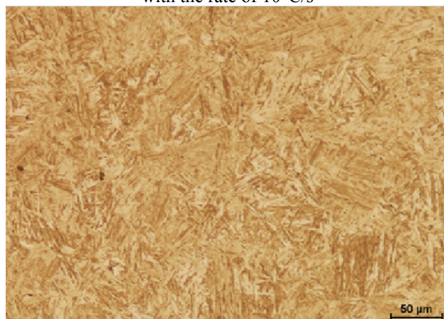
Figure 8. Martensitic structure of the specimen made of 30MnB4 steel after a deformation cycle cooled with the rate of 100°C/s
