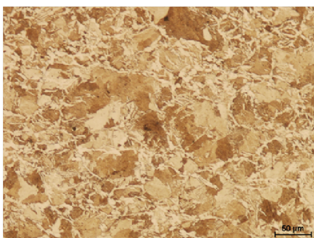
Figure 5. Ferritic-pearlitic microstructure of the specimen made of 30MnB4 steel after a deformation cycle cooled with the rate of 5°C/s
