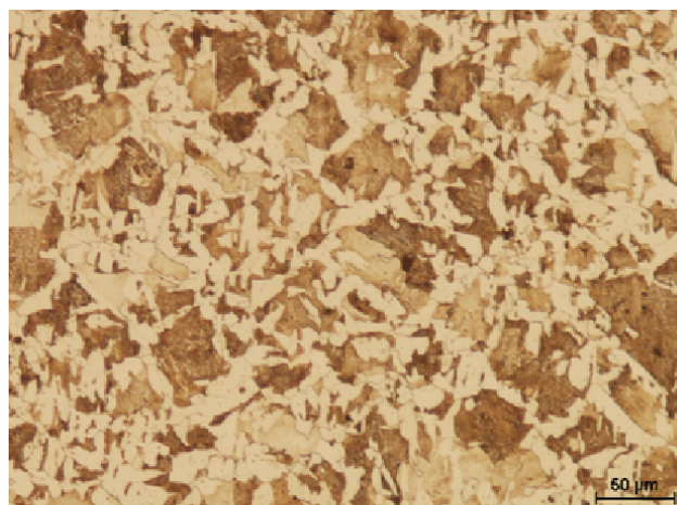
Figure 4. Ferritic-pearlitic microstructure of the specimen made of 30MnB4 steel after a deformation cycle cooled with the rate of 1°C/s
