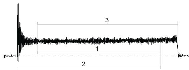
**Figure 1.** Recording and processing areas of the elastic force moment, being analyzed.
