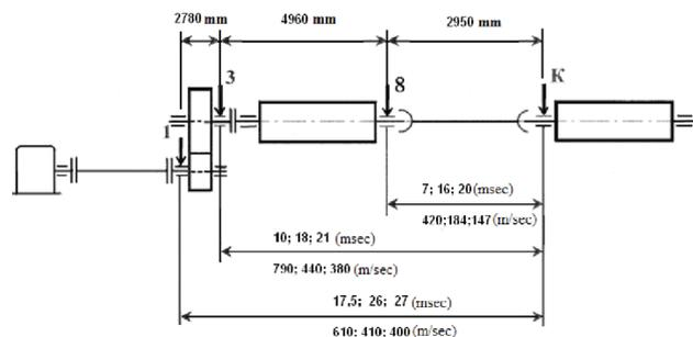
**Figure 6.** The measured values of the delay time of three areas and the estimated speed of the shock pulse passage of areas.
