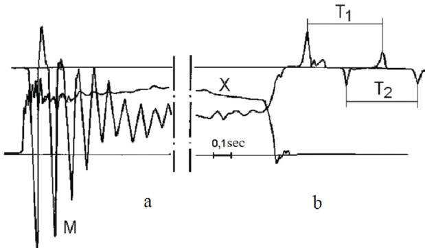
**Figure 5.** The transient in rollers drive line on the intermediate shaft between the engine and geared system (moment  $M$  of elastic forces) and the stand elastic system (deformation  $X$  of housing post) at the capture (a) and after the output (b) of the band from the rolls.
