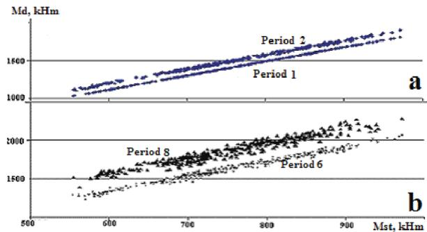
**Figure 3.** The calculated correlation fields: 1 - at the initial period of stand operation after the installation of spindles with new livers (minimum clearance), 8 - before the replacing of spindles with worn livers (wear and gaps are maximum).
