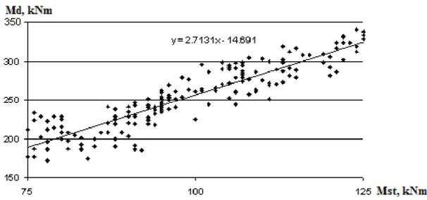
**Figure 2.** Correlation field  $Md$ ,  $Mst$  as measured in the stand 6 of mill 1680.
