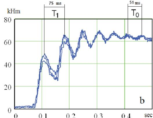
**Figure 4.** The actual difference in  $T_1$  and  $T_0$  periods between the time the first two peaks of the elastic forces moment (a) and the engine (b) from the results of measurements.
