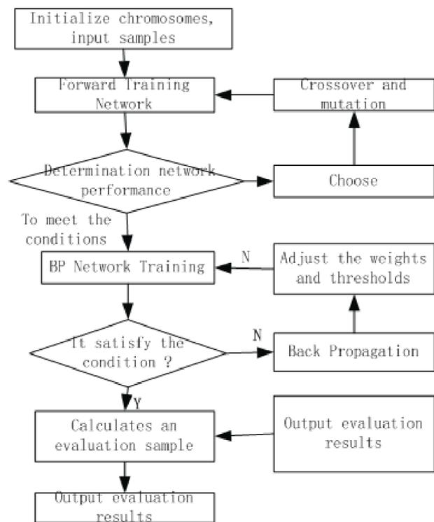
**Figure 3.** Genetic Algorithm optimization BP neural network processes
