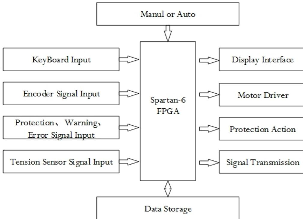
**Figure 1.** Hardware block diagram of system
