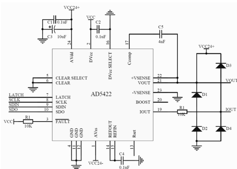
Figure 2. Circuit diagram of AD5422
