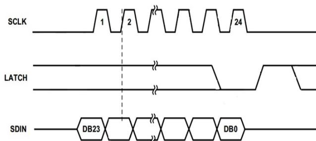
Figure 3. Timing diagram of SPI
