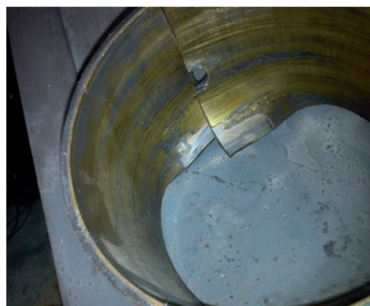
Figure 1. External and internal surfaces of the main support bearing insert in module No 9, the insert is out of order due to working roll shaft damage
