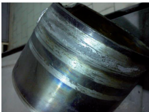
Figure 1. External and internal surfaces of the main support bearing insert in module No 9, the insert is out of order due to working roll shaft damage
