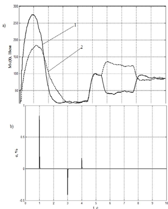
**Figure 3** Modeling results of identification of the static moment on the working rolls of the break-down mill during unilateral slip on the lower working roll: a) identified static moments of working rolls (1 – lower roll, 2 - upper roll) while loading the lower roll,  $\text{Hc}\cdot\text{m}$ ; b) error of static moment identification, %
