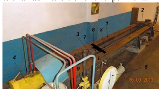
Figure 2. Fragment of the rope 28-G-V-N-R-1770 parameters researches (GOST 2688-80) of the drilling rig feed SBSH-250 of the tensile machine "ALFRED AMSLER and Ko": 1 – bed; 2 – back motionless poppet; 3 – movable headstock; 4 – the tension hydraulic cylinder; 5 – a scale for loading control; 6 – motionless measuring plank for the rope stretching control relating to the hanger 7 connected to hydraulic cylinder 4 rod; 8 – the rope under test; 9 – crane of pressure regulation in a hydraulic cylinder; L – distance between a measuring plank 6 and hanger 7, which was measured by means of beam compass.
