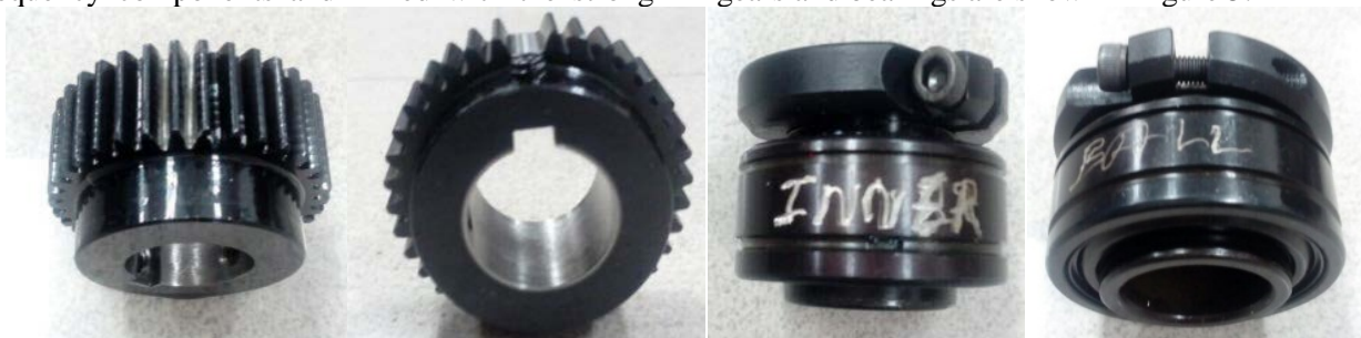
(a)Root crack fault
