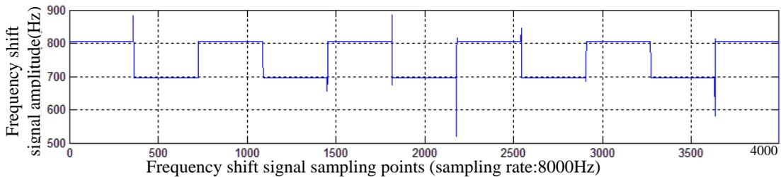
**Figure 4.** The transformation result of the upper/lower side frequency by using the method of this paper to analyze Figure 3
