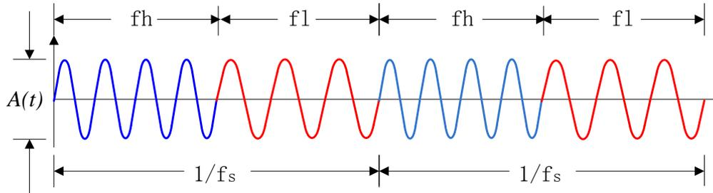
Figure 1. Frequency shift signal diagram
