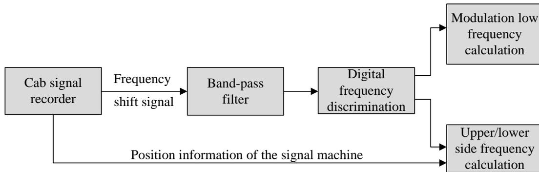
**Figure 2.** Block diagram of frequency shift signal frequency detection principle
