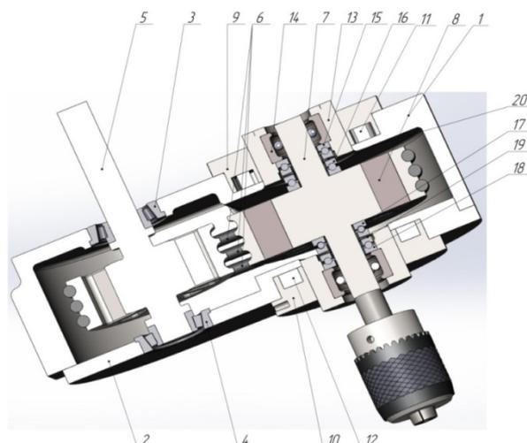
**Figure 1.** Device for vibrational drilling 1 – body 2 – housing cover; 3,4 – bearings; 5 - input shaft; 6 - flexible coupling; 7 - output shaft; 8 – magnets; 9, 10 – magnetic bodies; 11,12 – magnets; 13 – screw; 14 – bearing; 15,16,17,18 - axial bearings; 19,20 - springs
