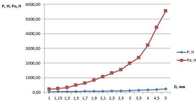
**Figure 2.** Dependency diagrams of critical load and axial force for the diameters from 1 to 5 mm during drilling: P – critical force during drilling;  $P_o$  –axial force during drilling.
