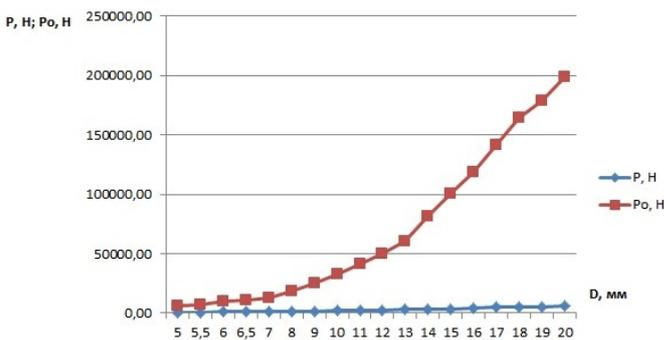
**Figure 3.** Dependency diagrams of critical load and axial force for the diameters from 5 to 20 mm during drilling: P – critical force during drilling;  $P_o$  –axial force during drilling.
