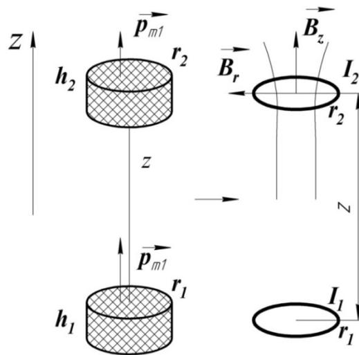
**Figure 4.** The scheme of interaction of permanent magnets
