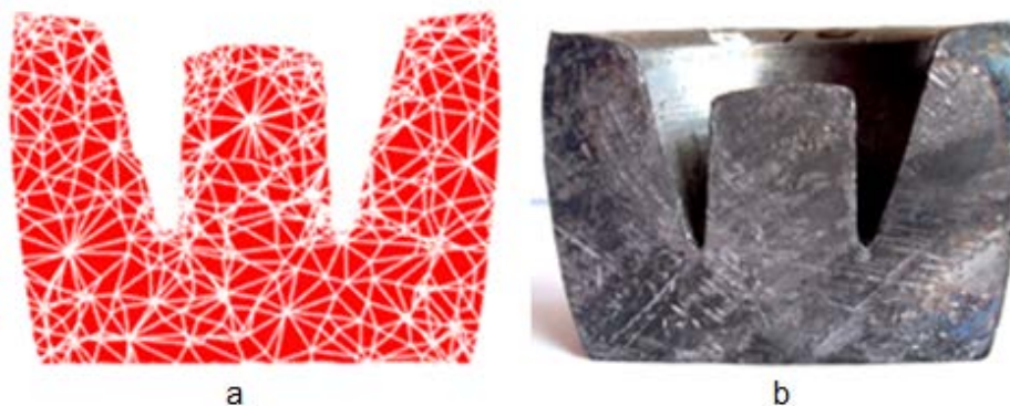
Figure 3. The comparison of geometry of samples obtained after the first stage a – the appearance of a sample obtained by the way of mathematical simulation; b – the appearance of a sample obtained by the way of experiment
