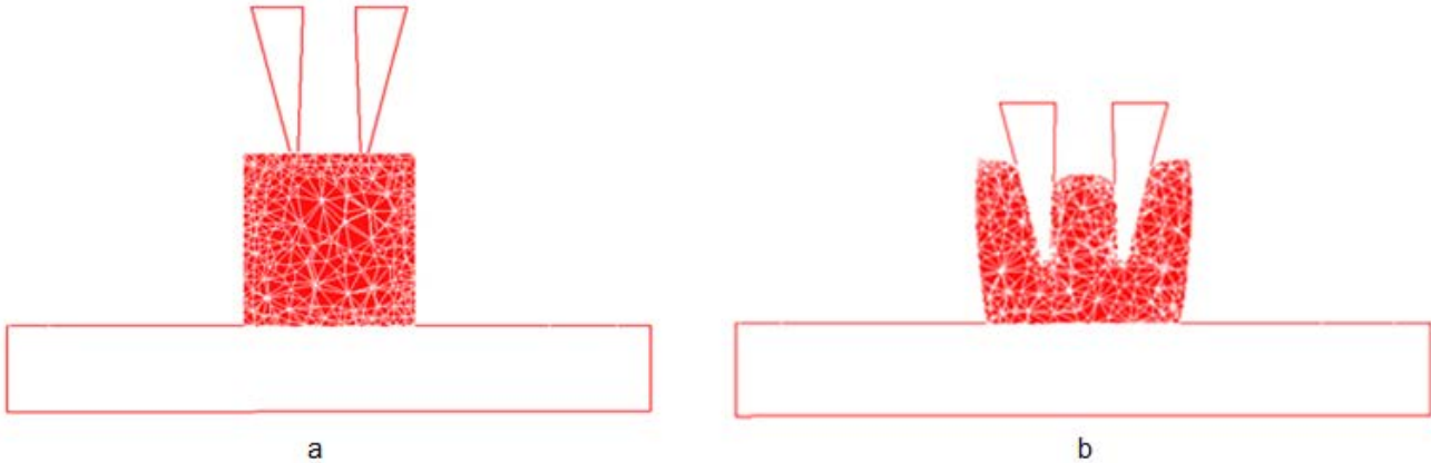
Figure 2. The mathematical simulation of the “cut-in ring” penetration
