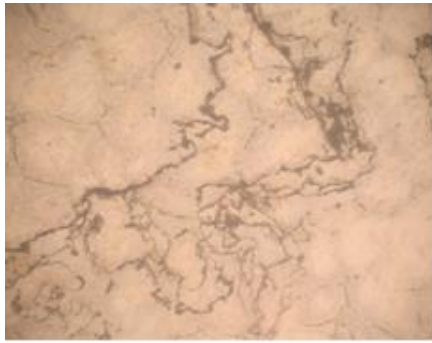
Figure 2 Coarse scabs in samples of ML10 alloy with additive 1.0 % Sc, x100.
