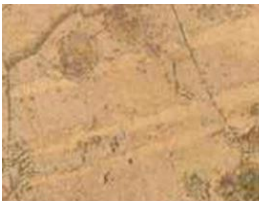
Figure 6 Inhomogeneous separation of secondary intermetallide phase in the sample of ML10 alloy after prolonged keeping (1252 hours, \sigma_r = 80\text{MPa} ) at the temperature 150°C, \times 750 .
