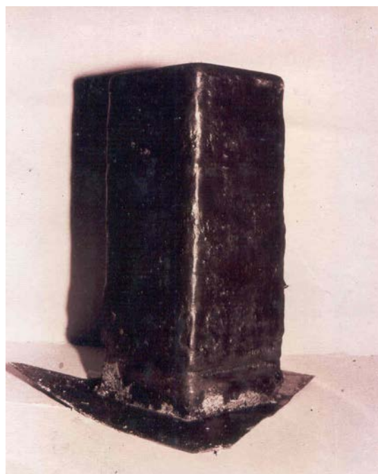
Fig. 5b ESR ingot of square cross section produced by using redesigned mould
