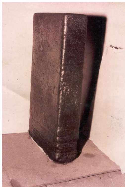
Fig. 5a ESR slab produced by using produced by redesigned mould
