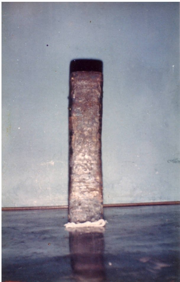
Fig. 4 ESR ingot produced using redesigned mould in trial runs
