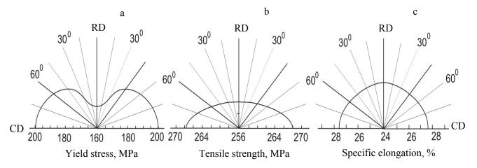
**Figure 2.** Anisotropy of yield stress (a), tensile strength (b), specific elongation (c) of AZ31 sheets after hot rolling and recrystallization annealing
