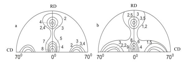
Figure 1. Pole figures (0002) of AZ31 sheets after deformation: a - 1 cycle; b - 8 cycles of sign-variable bending
