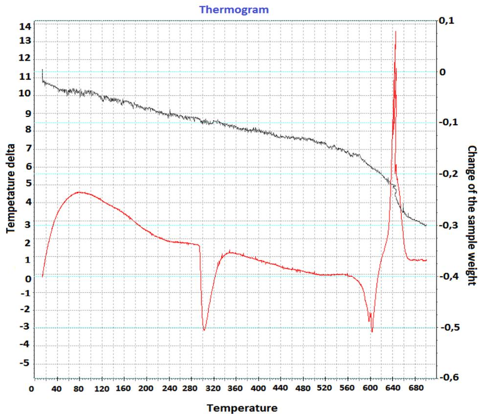
Figure 1. The thermogram of potassium perchlorate decomposition without catalysts
