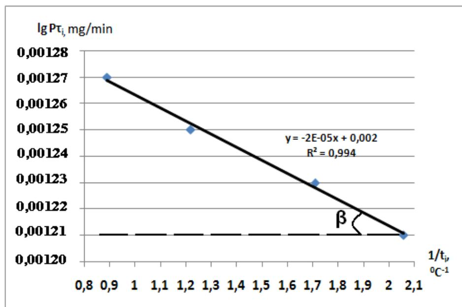
**Figure 4.** The semi-logarithmic dependence of the change of decomposition speed of the mixture, which consists of PP and manganese oxide from the inverse temperature
