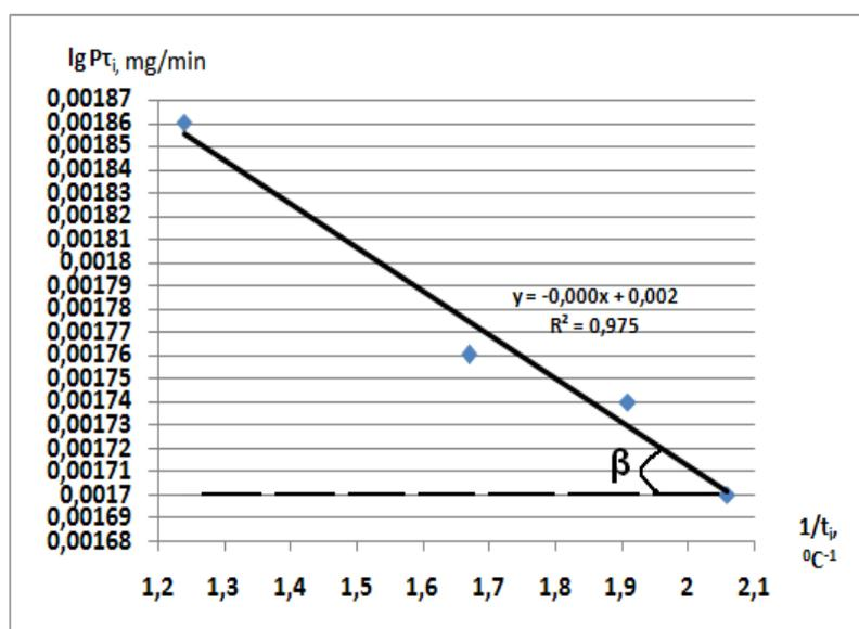
**Figure 3.** Semi-logarithmic dependence of the change of PP decomposition speed on the inverse temperature
