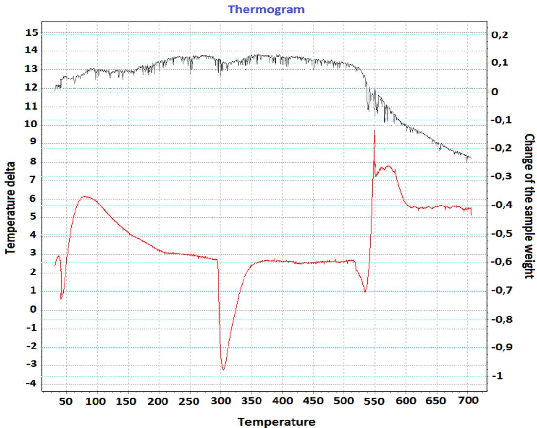
**Figure 2.** The thermogram of the decomposition of potassium perchlorate mixture with catalyst manganese oxide
